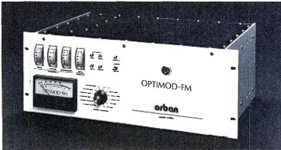
Orban's Optimod-FM audio processor
